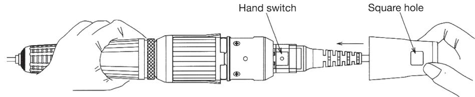
9. While the power is off, plug handpiece into controller. Please speed up gradually from minimum RPM and make sure nothing is abnormal with behavior.
