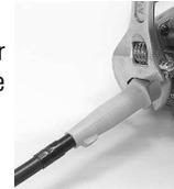
Loosen set screw on the flexible shaft motor coupling and slide shaft off the motor shaft.
