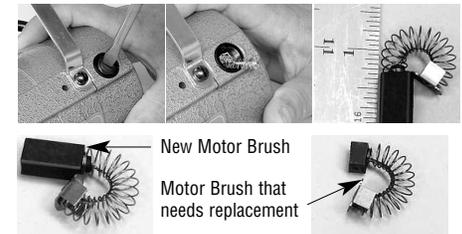
brushes match the contour of the armature when replacing them. Be sure to replace both motor brushes even if one of them is less worn than the other. To remove dirt and dust buildup, when motor brushes are checked or replaced, compressed air should be blown through the motor.
