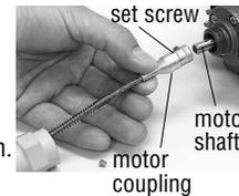
3. Grease shaft prior to putting on the sheath. (See Lubrication instructions on page 6.)
