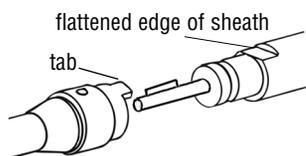
Unlike other Foredom Handpieces, the H.9D handpiece has a tab on the end where it connects to the shaft and sheath (see drawing). The tab slides over the flattened edge on the sheath. **The H.9D will not fit other Foredom sheaths.** However, other handpieces can be attached to the PowerGraver shaft for slow speed jobs.
