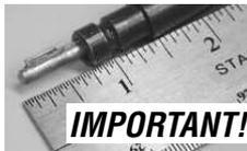
**exposed tip (handpiece end) of the inner shaft so that it extends 3/4" (19mm) beyond the outer sheath, as shown above. This is done by moving the sheath in or out of the motor connector (motor end) as shown above right.**
