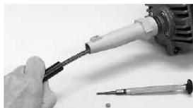
4. Apply a very light coating of lubrication to shaft starting at the top and working downward to
