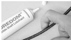
about one inch from the handpiece end. Apply grease with your finger tip or small brush. Don't overdo, apply a light film of grease. Once the machine is running, the shaft itself will spread the grease. If too much grease is applied, the excess will work its way into the handpiece and eventually seep out between the handpiece and sheath. For this reason, apply a bit less near the handpiece end of the shaft.
