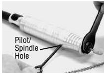
**To insert accessory:** insert shank as far as possible into the collet. Tighten chuck nut. Test for a secure hold by pulling on accessory. Remove wrenches. To release an accessory, follow the same steps. Accessories can be released when chuck nut is loosened. If accessory does not run true, loosen chuck nut, rotate accessory, and retighten.
