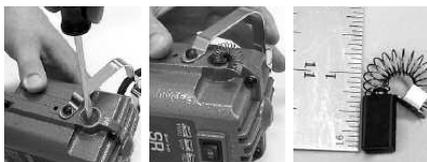
Motor brushes should be checked for wear periodically. When new they are approximately 3/4" (19mm) long. Replace them when they have worn to 1/4" (6mm). To remove brushes, disconnect motor power cord and unscrew the brush caps. Remove the worn motor brushes, replace with new motor brushes, and screw motor brush caps back on. Be sure to replace both motor brushes even if one of them is less worn than the other.
