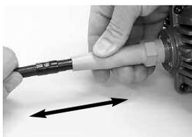
**5.** Slide sheath over flexible shaft with plain fitting directed toward the motor and into the motor connector. (Each end of the sheath has a metal fitting. One is plain, the other has a groove around it to fit the handpiece.)
