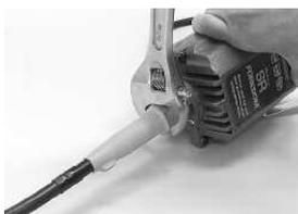
Loosen set screw on the flexible shaft motor coupling and slide shaft off the motor shaft.
