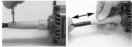
When the correct adjustment is made, re-tighten the set screw in the motor connector and re-attach handpiece onto the flexible shaft.
