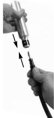
To verify this, insert and tighten an accessory into collet or chuck, turn on control to a low speed and observe that the accessory rotates smoothly.
